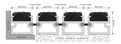
Structure in robust PVC shock-proof and scratch-proof tubular profiles joined by thermoplastic high-strength channels perforated or closed. Non-slip certification R-12 according to DIN 51130 regulaton. Space between the slats 7 or 4 mm. Lining of rich technical needle punched velvety appearence. Thickness 25mm. c.a.
