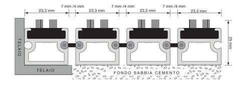
Structure in robust PVC shock-proof and scratch-proof tubular profiles joined by thermoplastic high-strength channels perforated or closed. Non slip certification R-13 accorfin to DIN 51130 regulation. Space between the slats 7 or 4 mm. Lining of monofilament tufts of nylon. Thickness 25mm. c.a.
