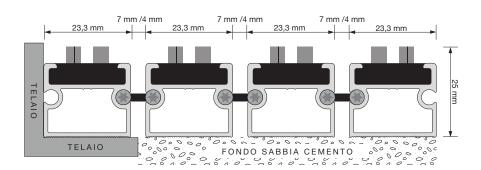
Structure in robust tubolar aluminium wires joined by thermoplastic channels high-strenghts buttonholes or closed. Non slip certification R-13 accorfin to DIN 51130 regulation. Space between the slats 7 or 4 mm. Lining of monofilament tufts of nylon. Thickness 25mm. c.a.
