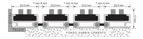
Structure in robust PVC shock-proof and scratch-proof tubular profiles joined by thermoplastic high-strength channels perforated or closed. Non slip certification R-13 accorfin to DIN 51130 regulation. Space between the slats 7 or 4 mm. Lining of monofilament tufts of nylon. Thickness 17mm. c.a.
