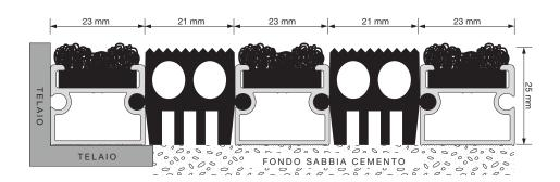
Structure in strong tubolar alluminium profiles joined by a laminated rubber EPDM profile. No space between the slats (closed mat). lining in rich technical needle-punched with almondy appearance. Thickness 25mm. c.a.
